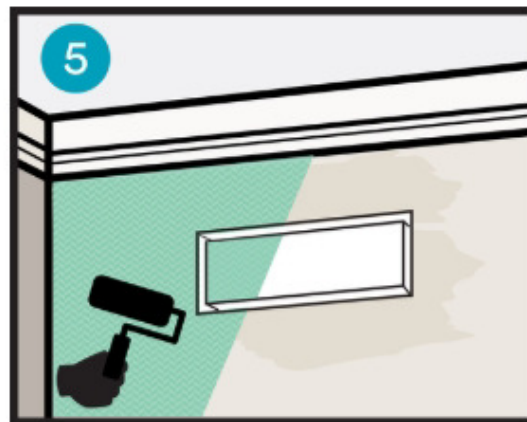
Paint walls and surface of tray insert.
